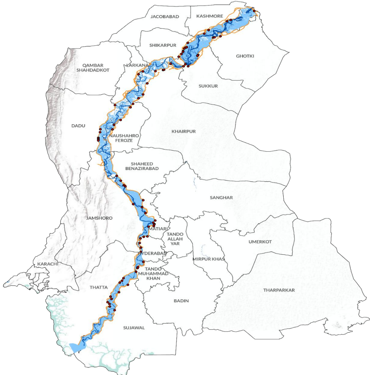
Figure 2.7.1 Vulnerable Locations of River Embankment
