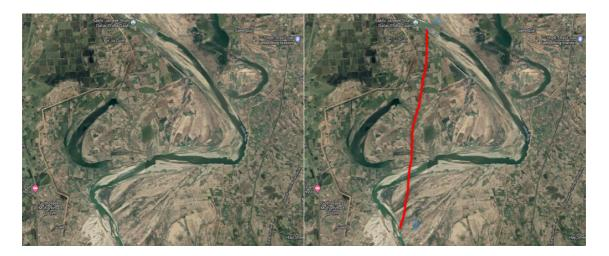
Once path A to B has been developed, then river in normal condition will flow in this path. However annual or bi-annual cleaning of this path will be required by removing the sediments/clay deposit in this path. Special boats will be required to carry out this task by excavating the sand/clay beneath the river and put it on its sides. This solution may minimize damaged losses (life and material) due to breaching scenarios.
